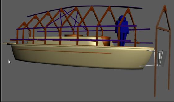
The 9 truss components are basically all cut the same with exception of the sides. The side lengths are critical since they dictate the overall width of each truss. The following table shows the required lengths of the two side pieces for each truss.
