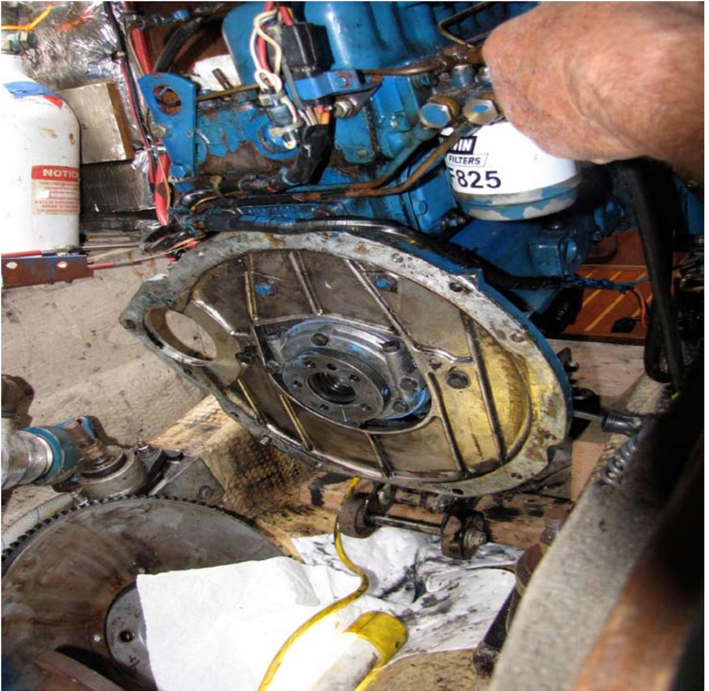
**Remove flywheel, exposing engine shaft coupler. Note the oil seal housing immediately behind the mounting flange,**
