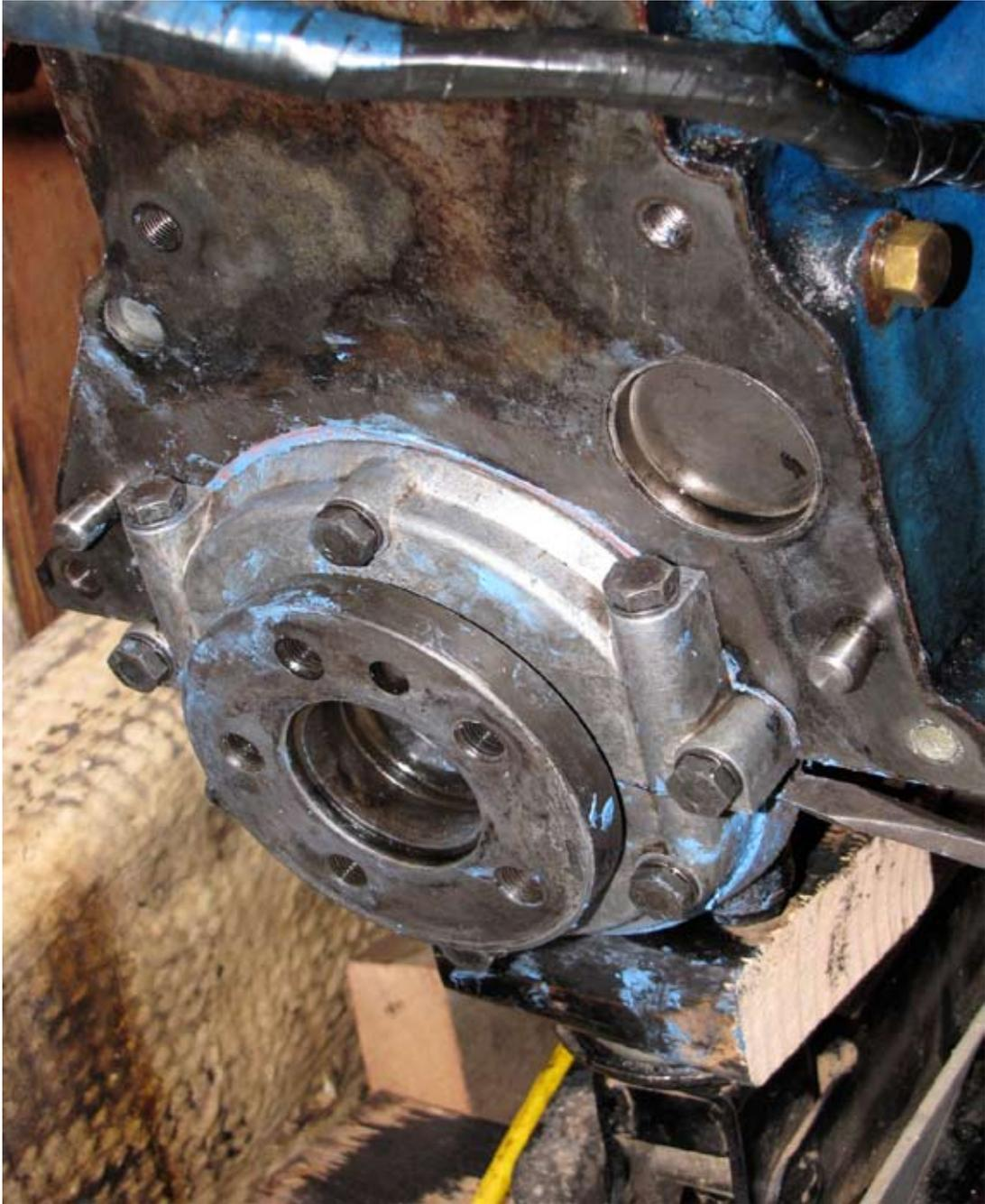
**New oil seal and mount bolted to engine casting; oblique view.**
