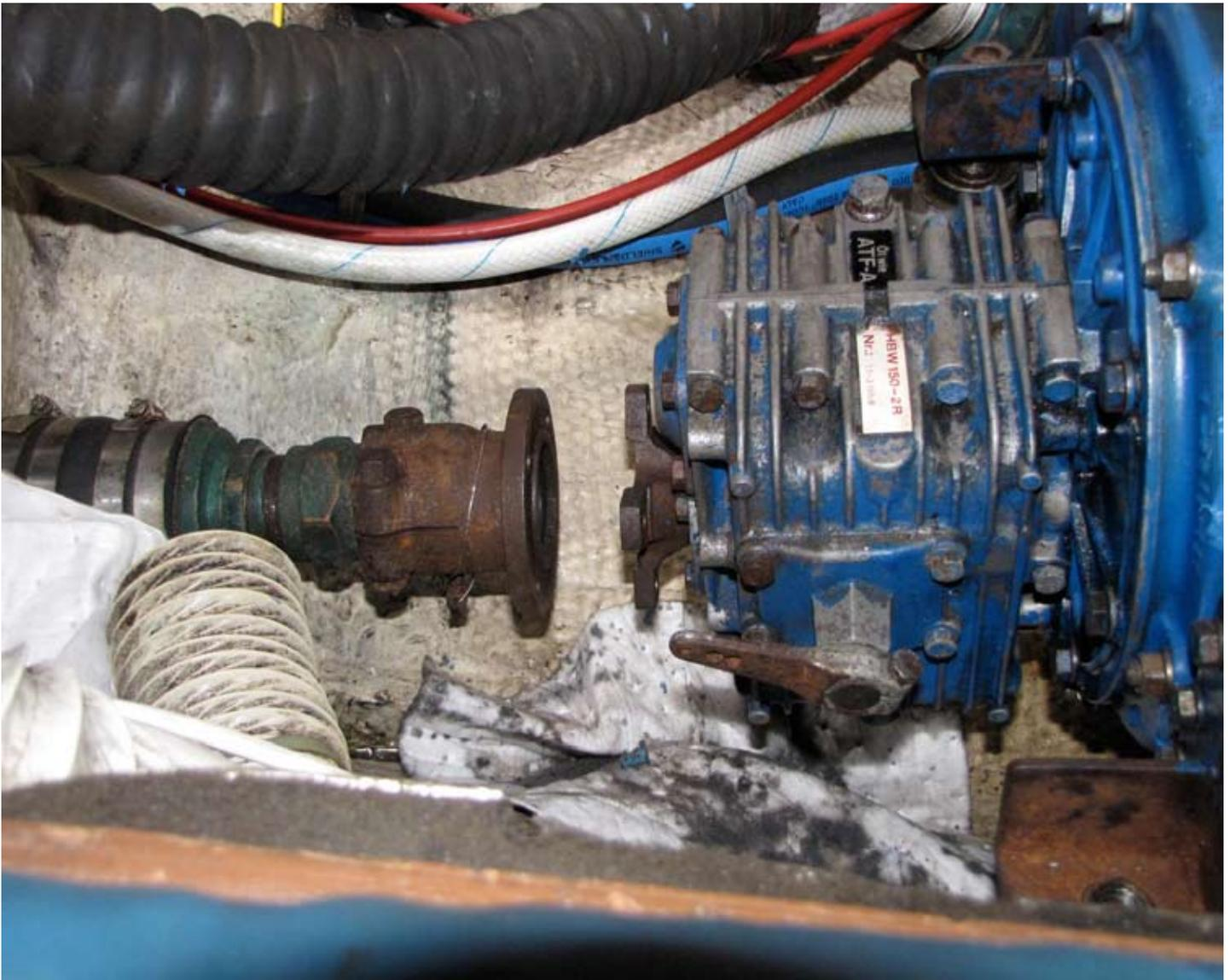
**Step 1: Disconnect propshaft from engine, and push as far back as possible. This leaves a gap of 1.5" - sufficient to remove gearbox**
