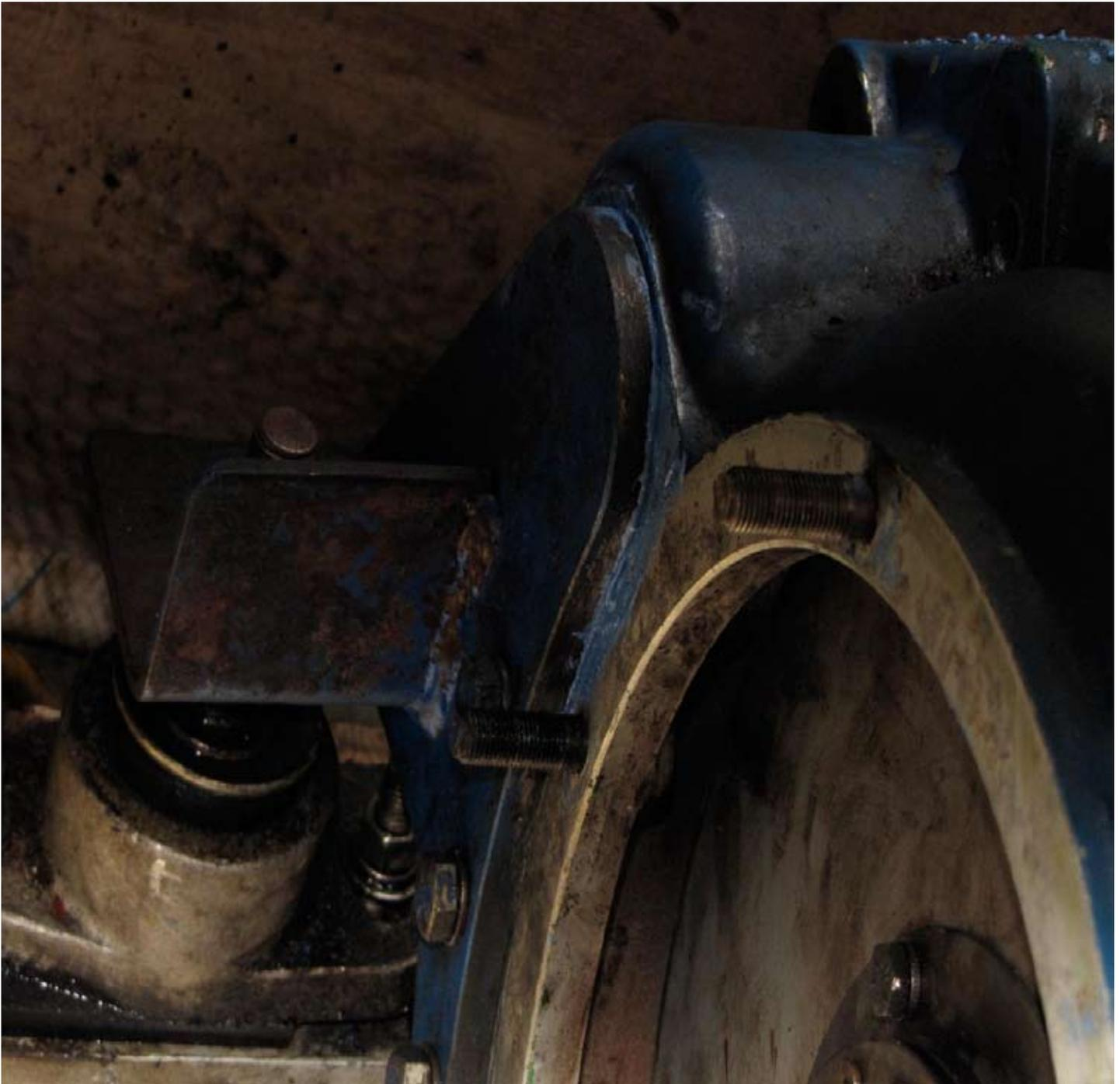
**with the engine raised it is possible to easily unbolt the bracket shown in this image that attaches engine to engine mount. Remove both port and starboard bracket**
