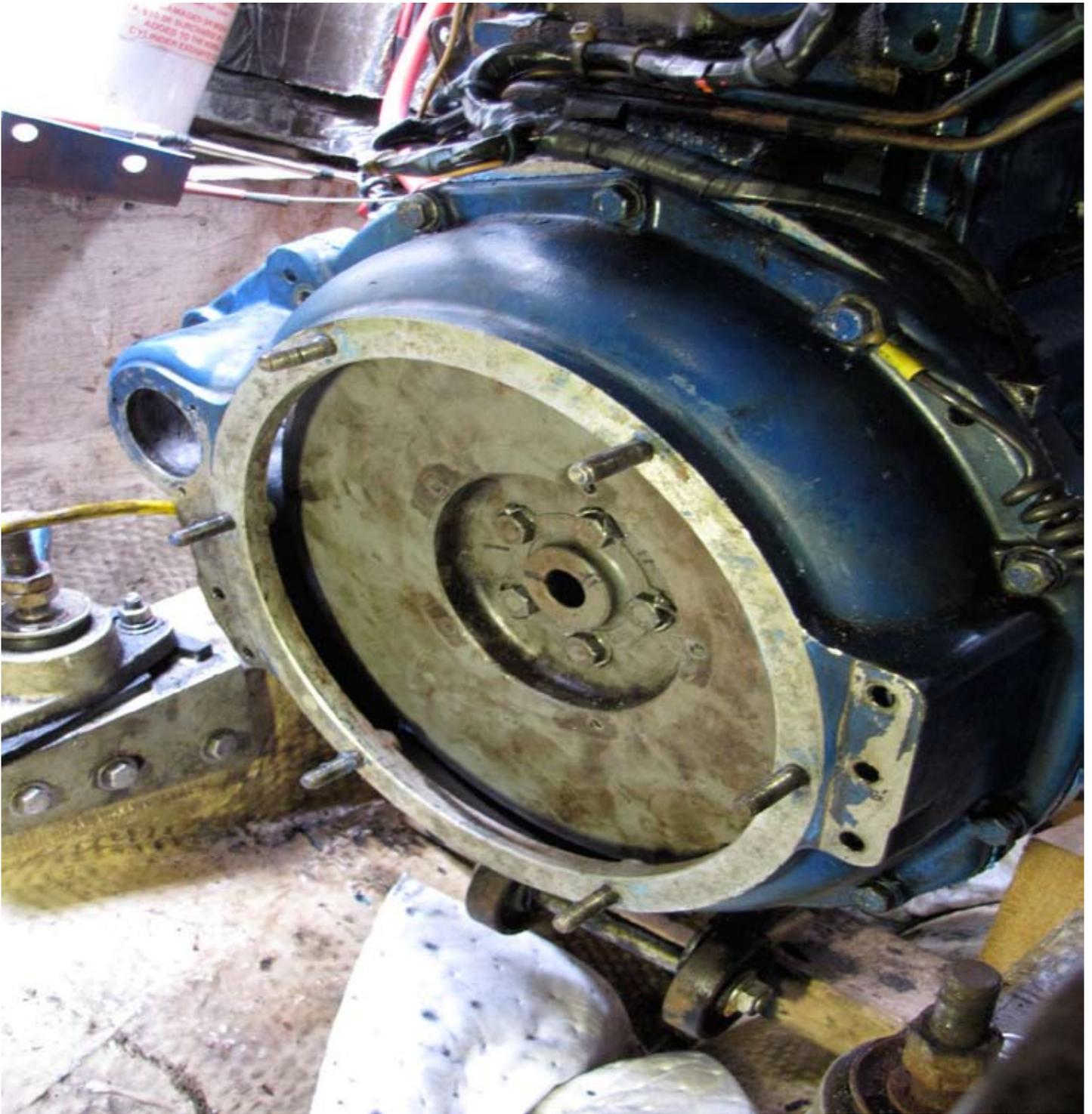
**Coupler removed showing five bigger bolts attaching flywheel to engine drive shaft**
