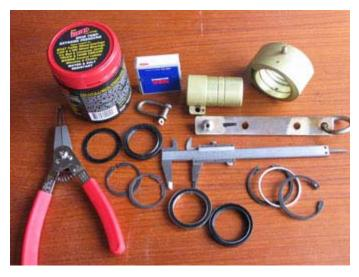
N42 Bearings - 80x50x10mm deep groove - NSK #16010 or equivalent -
