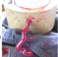
After assembling with new bearings and seals with copious "wheel bearing" grease, the excess was forced out through these holes. I then blanked them off with 6mm machine screws. My
