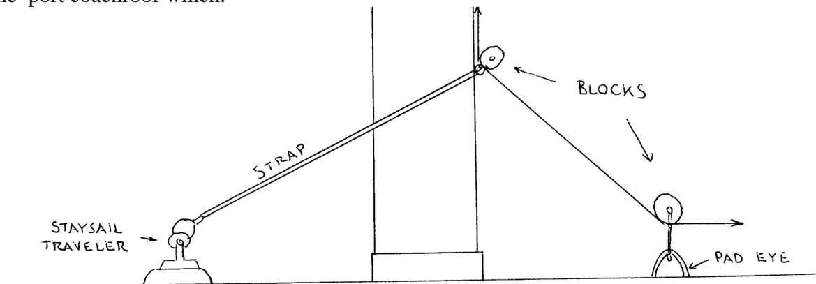
4. Ron Gemme, "RISE", has a Nicro Fico traveler and found he could not mount an adequate control line system on the factory installed padeyes at the ends of the laminated teak bar. Ron removed the large padeyes and installed special blocks designed to hold two cheek blocks. The sheaves on the traveler car were replaced with beckett blocks yielding a 3:1 purchase (especially helpful for Marilyn).
