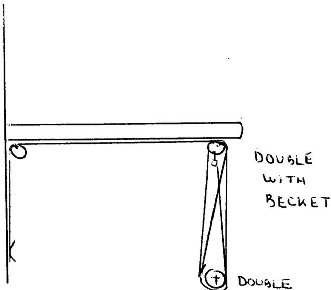
2. Lee Cross, "LEYENDA", put an eye bolt in the davit deck securing plate and uses it for a turning block for his running back stays; a spinnaker sheet block; and for wire safety lines running up forward.
